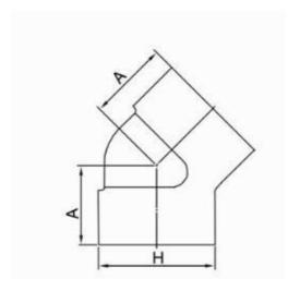
High Press Threaded 45 Degree Elbow
