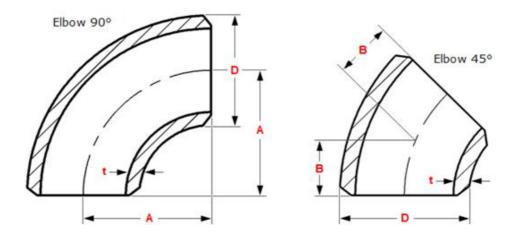
ASME Large Caliber Pipe Fitting Elbow
