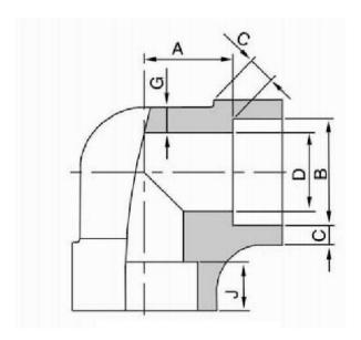
High press pipe fitting elbow
